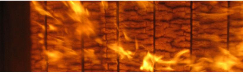
A solid timber element burns extremely poorly, it will only char slowly on its surface – it is very difficult to set a thick beam on fire. This charring acts immediately as a natural fire protection and ensures that the wood will burn very poorly. The structural integrity of a building is guaranteed even in case of fire as the core remains stable for a long time. Since the system uses wooden dowels, there is no risk that metal connectors could melt thus causing premature collapse.
