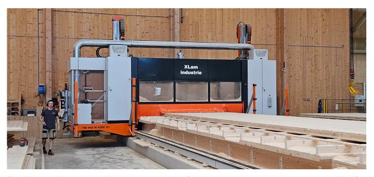
Techno Wood installed a portal robot at Xlam Industrie, equipped with a five-axis spindle including a tool changing system and an additional five-axis saw spindle.
