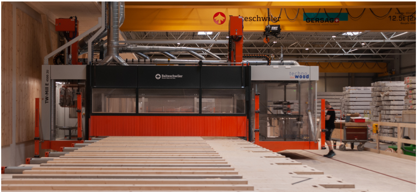
The TW-Mill E and TW-Mill M portals enable Balteschwiler AG to process a wide range of panels up to a thickness of 1.2 m
