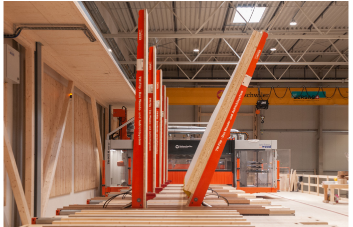
With the TW-Flip turning devices, panels weighing up to 7 tons can be turned safely.
