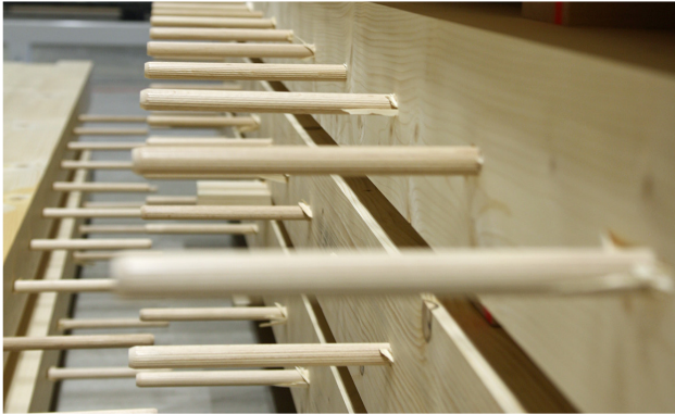
The laminated elements are connected with wooden dowels without any glue.
