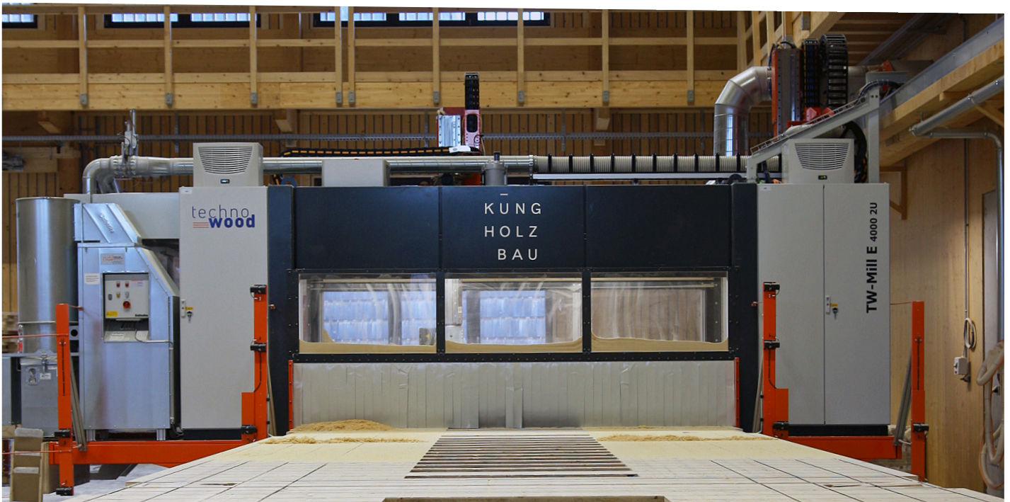
The dowel-laminated timber elements are processed on the new TechnoWood TW-Mill E 4000 2U system.
