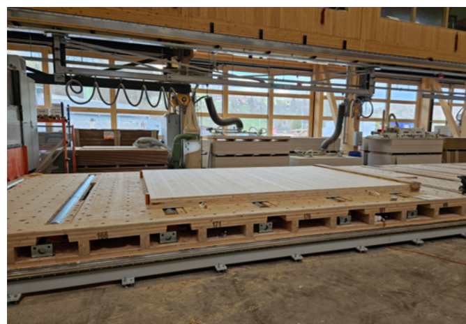
„HolzEcht“ wall elements made of adhesive-free solid wood are one of Schindler & Scheibling's specialties
