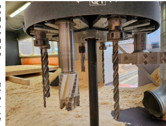
Xlam Industrie relies on Oertli tools from the Turbex and Castor series
