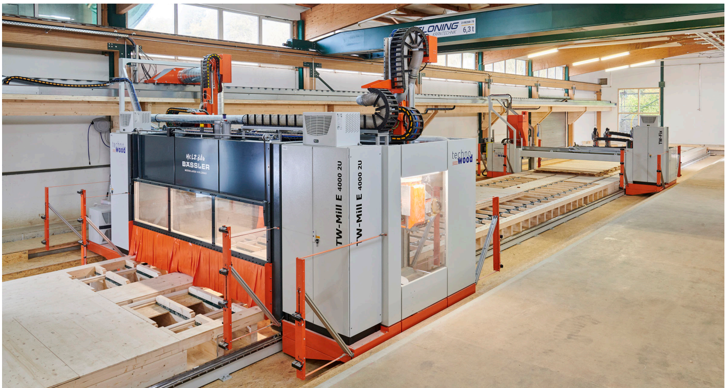
The compact production line consisting of the portal robot and the drilling and dowel portal - the system is designed for solid wood systems but also all common construction systems (Photo: Tom Philipp)
